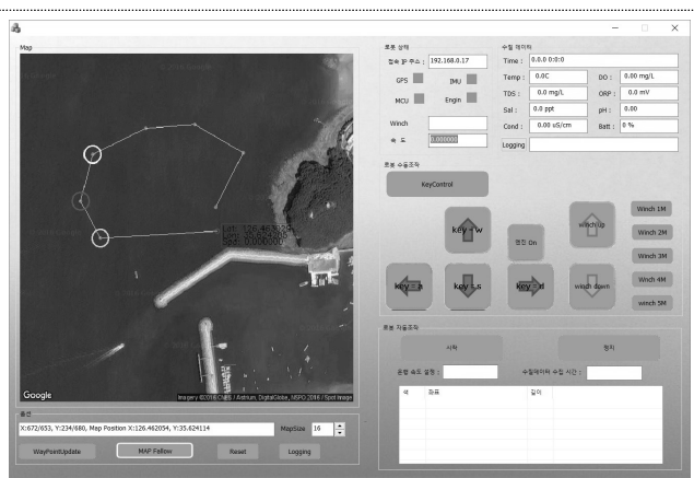
Fig. 7. GUI for Water Quality Surveillance according to user defined n Way point. (n=1, 2, ... l)
