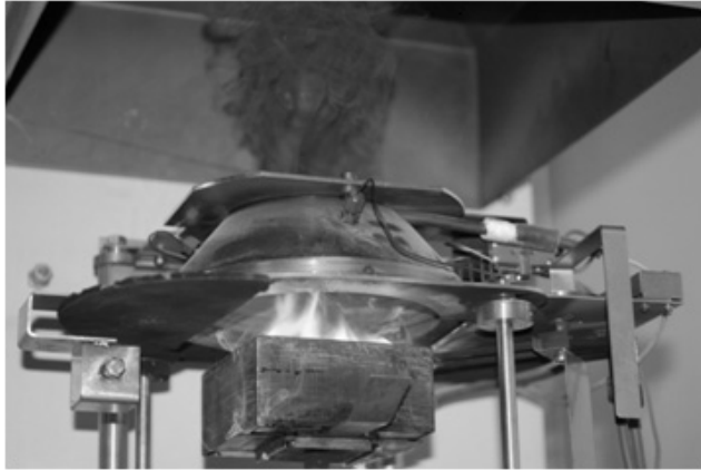
Fig. 1. Cone calorimeter test
