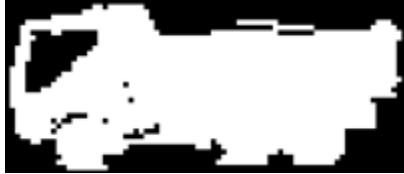
Fig.3 The 2D binary image after dilating and the image after contour segmentation
