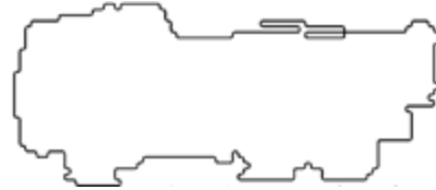
Fig.3 The 2D binary image after dilating and the image after contour segmentation
