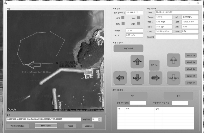
Fig. 9. Result of Measuring Water Quality at Defined Point (Green Rectangular)
