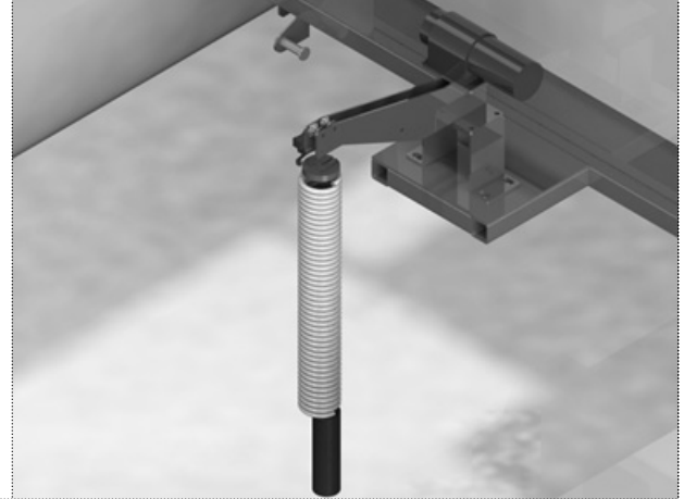
Fig. 2. Depth Control System of Water Quality Sensor
