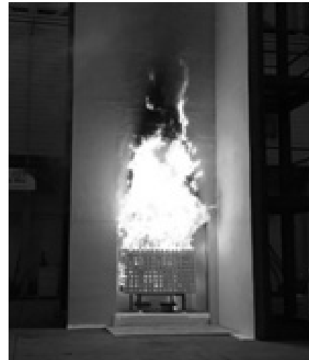
Fig. 3. BS 8414 Fire performance of external cladding systems. Test method for non-loadbearing external cladding system fixed to and supported by a structural steel frame
