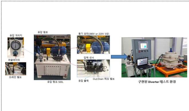
Fig. 3. Hydraulic Unit and PLC Control Unit and 7 1/4" Diverter
