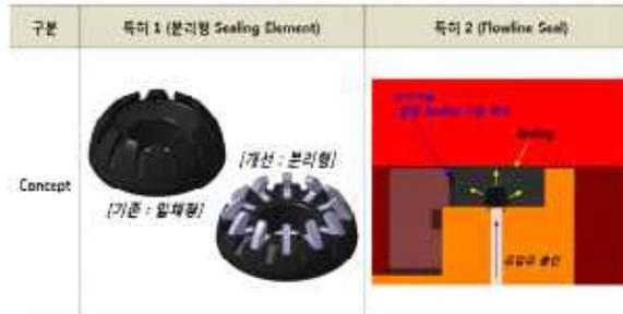
Fig. 4 Sealing Mechanism
