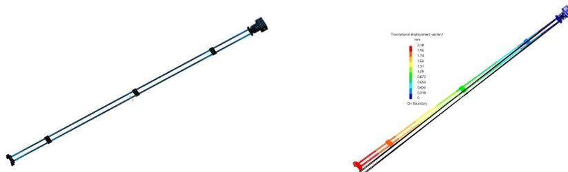
Fig. 4. Meshing of hammer bar and analysis result of displacement
