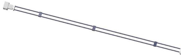
Fig. 3. Hammer bar assembly for nut pine threshing
