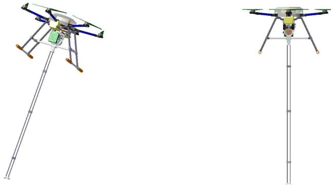
Fig. 2. Concept of hybrid drone system for nut pine threshing
