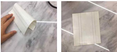
Fig. 1 Heating pad using carbon fiber
