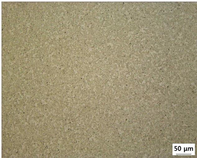
Fig. 3. Optical microscope of sintered tungsten material by acetone.
