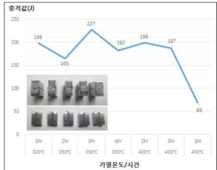
Fig. 2. graph of Impact test result
