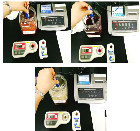
Fig. 4. Experimental view of pH, Brix and alcohol measurement
