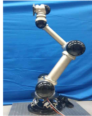
Fig. 2. Installation of a 6-DOF robot on the robot base platform
