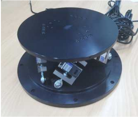
Fig. 1. Parallel-type robot base platform with 6-axis force/moment sensing
