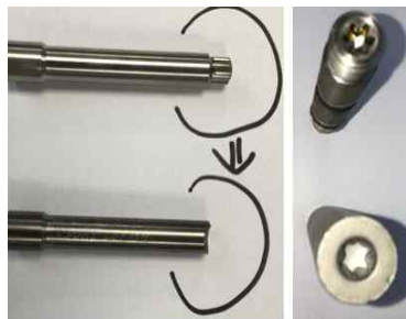
Fig. 1 Photograph of fractured punch
