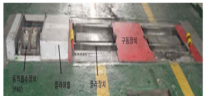
Fig. 2 System schematics of chassis dynamometer.
