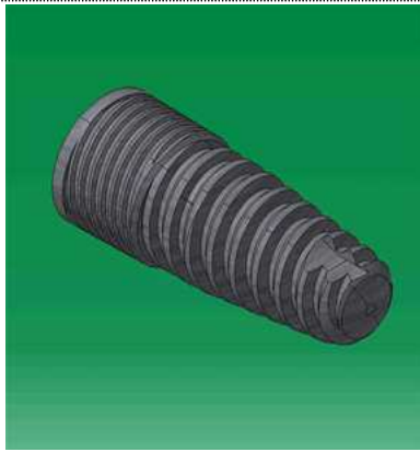
Fig. 1. a 3D a 3D model of typical micro-thread fixture
